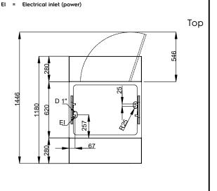
Electric Supply voltage: 220-240 V/1N ph/50/60 Hz Electrical power, max: 2.32 kW Water: Drain line size: 3/4" **Key Information:** N° of doors: External dimensions, Width: 800 mm 1180 mm External dimensions, Depth: External dimensions, Height: 1304 mm Net weight: 97.5 kg Shipping height: 1334 mm Shipping width: 840 mm Shipping depth: 899 mm Shipping volume: 1.01 m<sup>3</sup>
